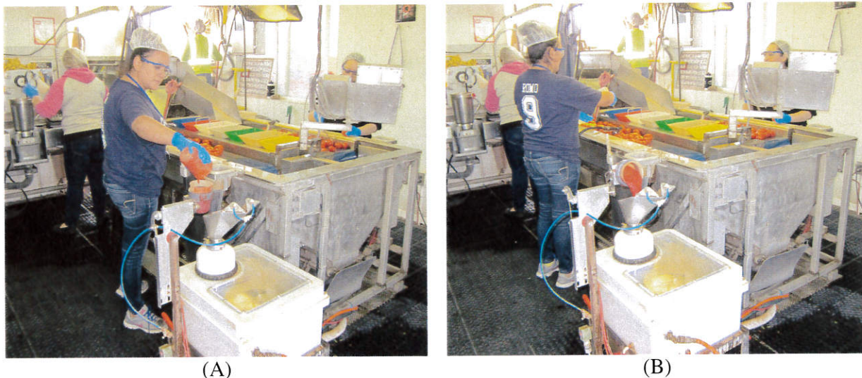
Figure 1. Photographic time sequence, showing the ruggedized color measurement system deployed at an inspection station. The picture in A shows the inspector in the foreground loading a new juice sample into the automatic pouring system. The picture in B shows the automatic pouring system transferring the sample into the internal viewing chamber for measurement as the inspector continues grading.
